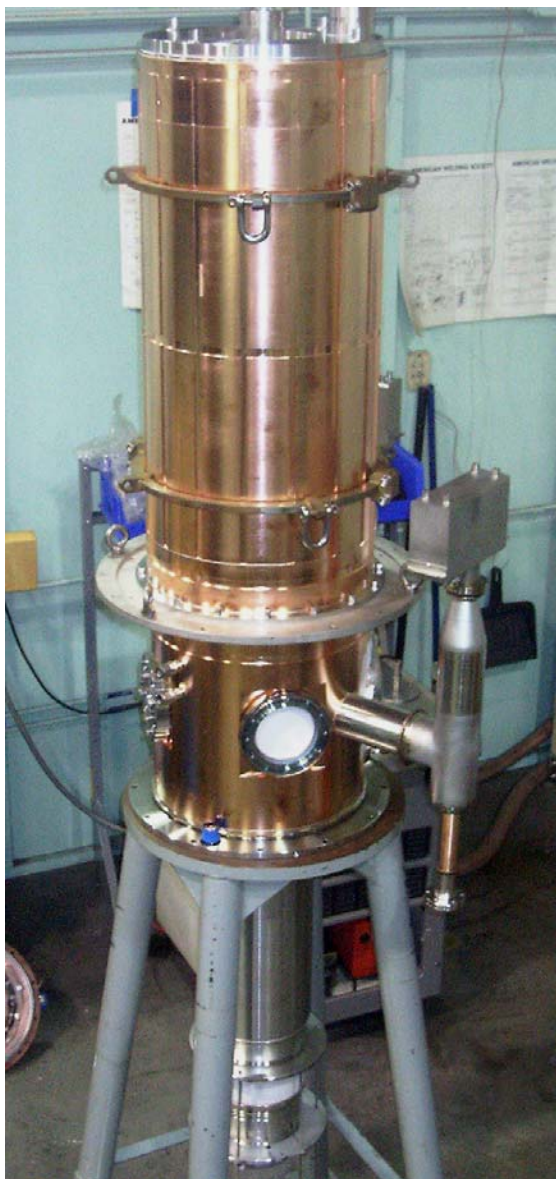
Figure 2. Photograph of the 1.5 MW 110 GHz gyrotron.
